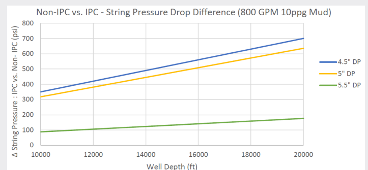
Figure 2 - Difference in String Pressure Drop Between IPC and Non-IPC Drill Pipe
