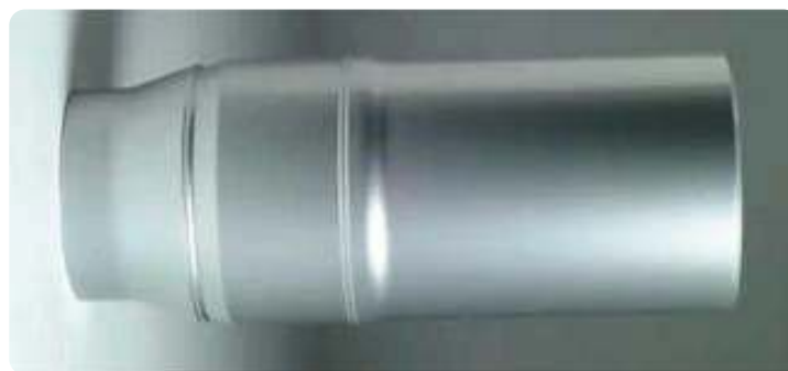
A dual-diameter tool joint is used to meet the two differing tool joint OD criteria, a balanced configuration, and required elevator capacity.
